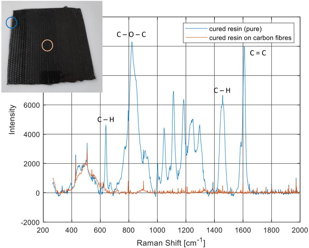
Figure 15. Baseline-corrected Raman spectra of a CFRP panel with amine-based epoxy resin system. While the peaks of the pure resin (blue) are clearly visible and can be identified with the help of the literature, the resin peaks collected on the fibres (red) are extremely weak and often cannot be distinguished from noise.
