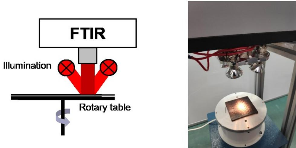
Figure 13. Laboratory setup for MIR spectroscopy of carbon fibre reinforced materials.
