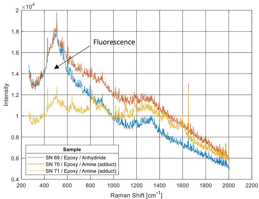
Figure 16. Raman spectra of CF samples with epoxy resin system that contain unspecific signals and a lot of noise. In addition, strong fluorescence is present.
