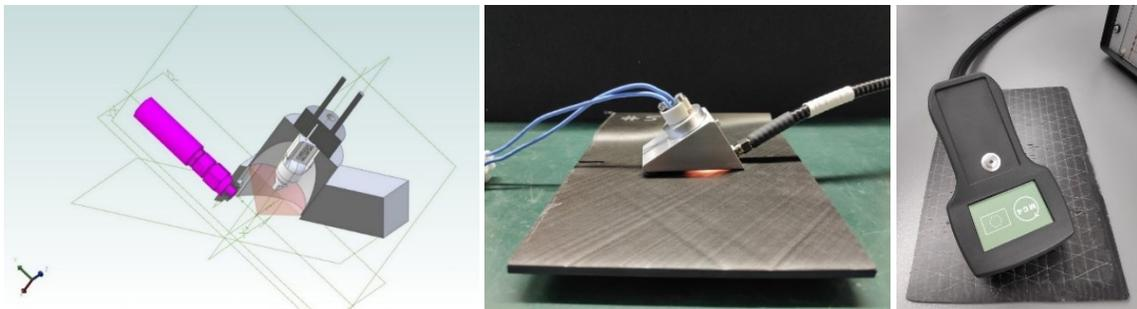
Figure 6. Left: 3D CAD drawing of the optimised reflection optics. Centre: Reflection optics (wedge-shaped component) during measurement on a CFRP plate. Right: Hand-held resin analyser (optics with housing); the measurement can be activated by pressing the circular button on the housing.
