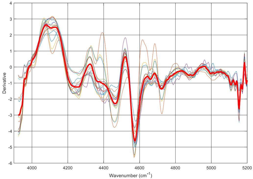
Figure 10. Post-processed NIR spectra (1. Derivative) of different amine-based epoxy resins on carbon fibres. The red, bold line represents the mean spectrum which was calculated by averaging all resin spectra. The legend with the sample descriptions has been omitted from the graph due to its length.
