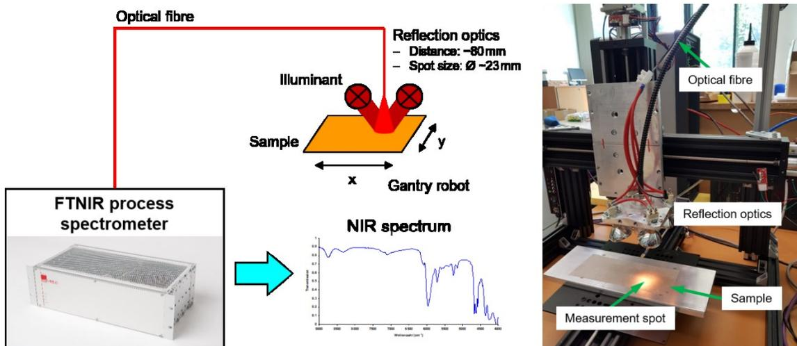
Figure 5. Stationary measurement setup for the FTNIR spectroscopic analysis of carbon fibre composite components in the laboratory.
