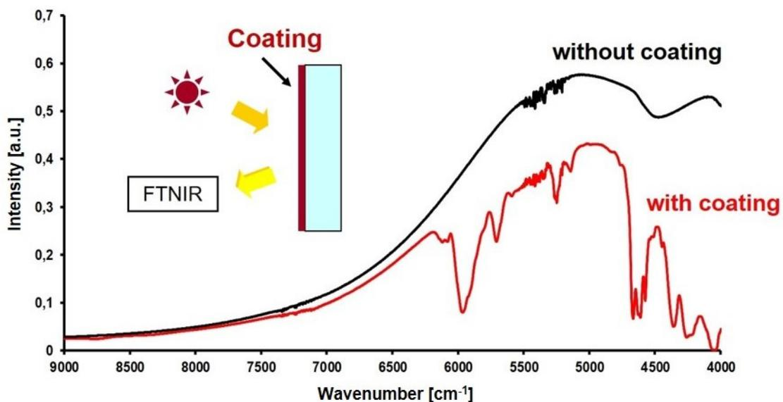
Figure 2. Principle of an IR reflection measurement shown on a metallic sample with and without resin coating. As the pure substrate reflects the incident light freely, a spectrum of the light source is measured. In contrast, the resin coating absorbs certain wavelengths of the incident light (indicated by drops in intensity), resulting in a characteristic resin spectrum.
