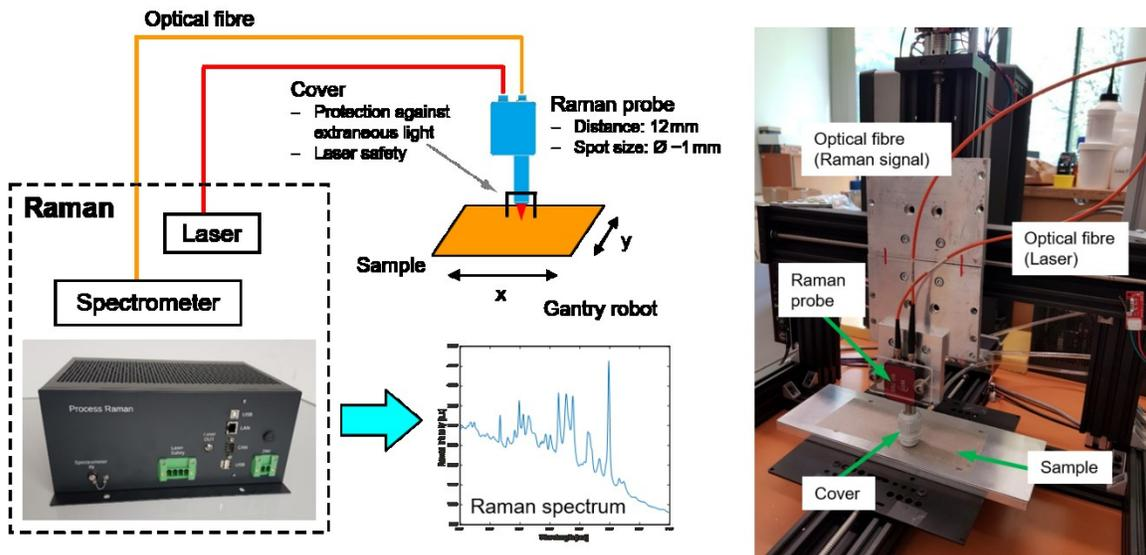
Figure 14. Measurement setup for the Raman analysis of carbon fibre composite components (small-scale implementation in the lab).
