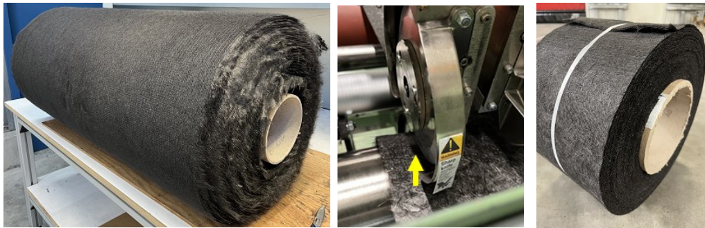
Figure 10: STFI rolls, to straight cut narrow tapes at CHOMARAT
