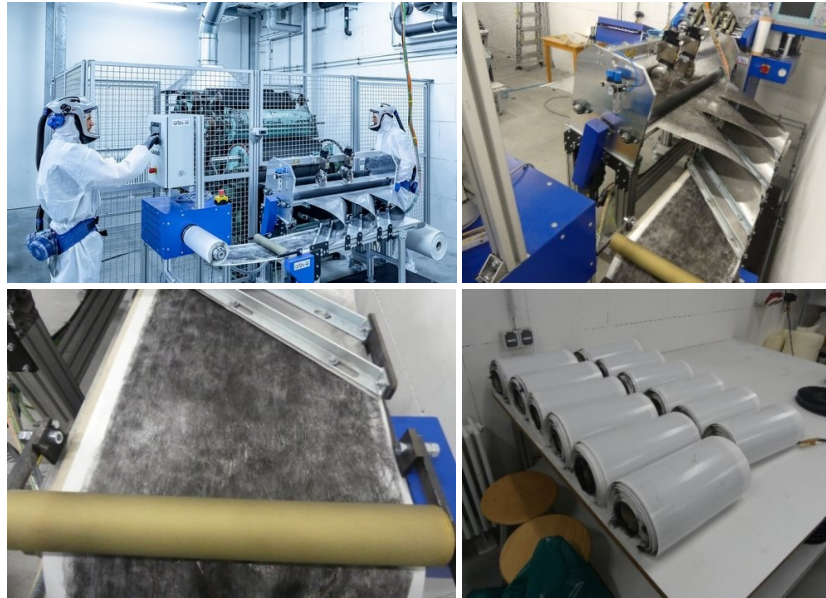
Figure 5: STFI nonwoven tape production from rCF
