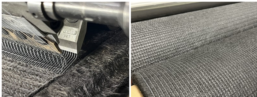
Figure 13: Detailed views of a rCF 0/90deg material (In the stitching area and on the winding device)
