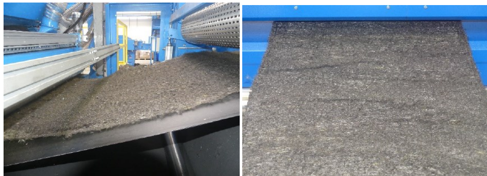
Figure 8: Illustration of wrinkles on a 200gsm STFI nonwoven with Gaiker fibres
