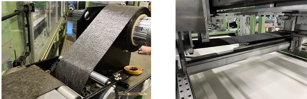
Figure 11: Offline station for unwinding and view of 90deg laying on the conveyor belt
