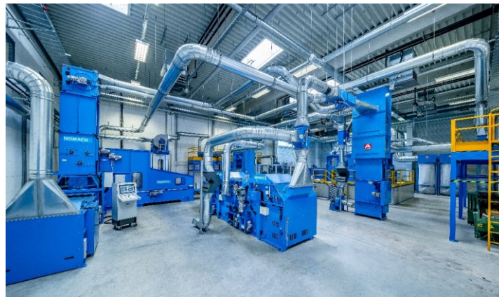
Figure 4: Scheme and photography of STFI carbon fibre nonwoven line
