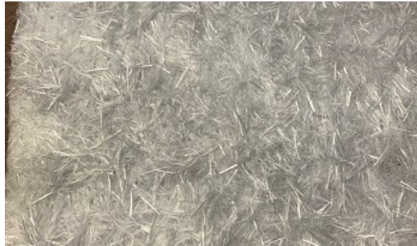
Figure 15: Example of a CSM structure with 18mm cut glass fibres from NCF waste
