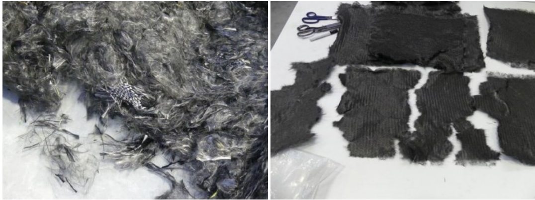
Figure 7: Initial evaluation of Gaiker fibres in STFI nonwoven processing (Failure with 50mm length)
