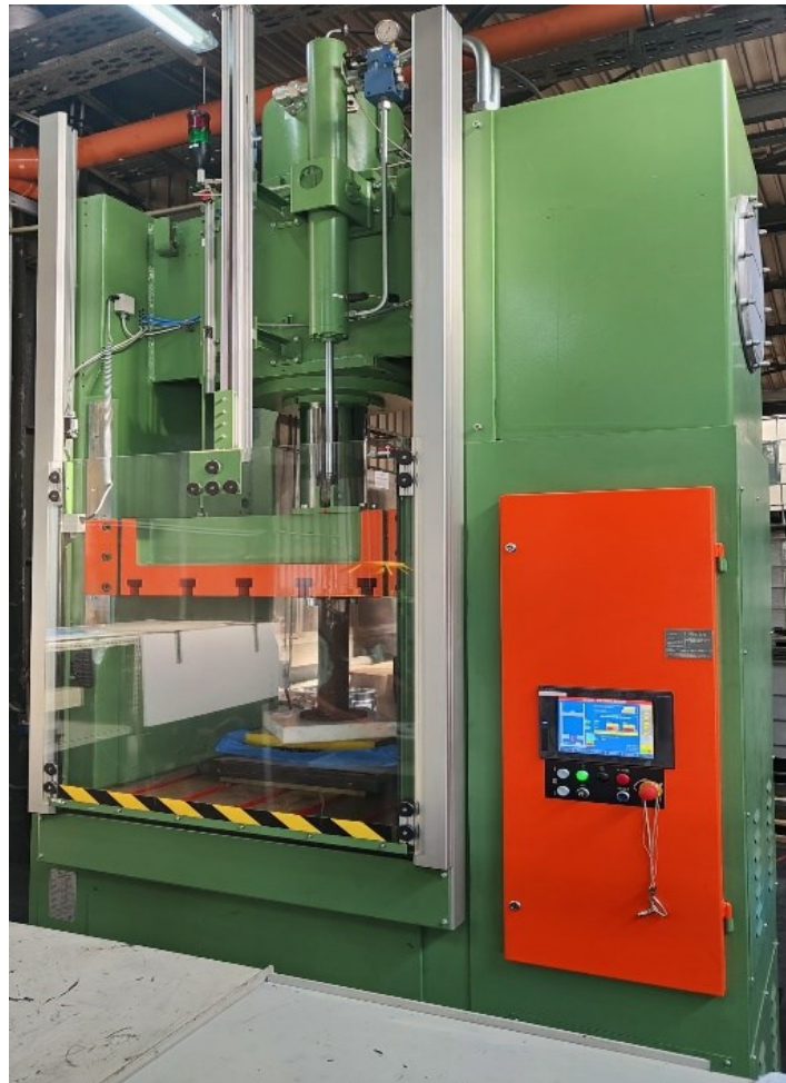
Fig. 4: Press for fabrication of components of joining collets.
