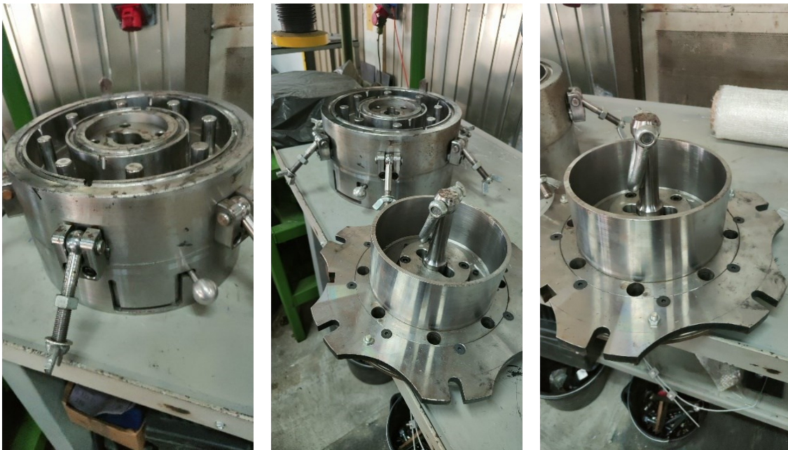
Fig. 6: Images of metal mould for joining collets fabrication
