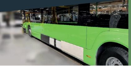
Jointly developed by VDL and CRC as part of the MC4 project, the bus side skirt integrates recycled composite materials from production waste into a new, high-performance component. Designed for public transportation, this innovative part demonstrates the potential of circular manufacturing, combining sustainability, efficiency, and enhanced mechanical properties.
