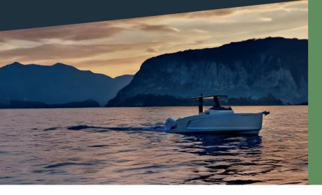
The SUN T-Top is a sustainable alternative for boats, made from recycled carbon fiber with the aim of reducing waste and minimizing environmental impact in the nautical industry. Developed by AMURA within the European MC4 project, this roof represents a major step forward in the circularity of composite materials in the nautical industry.
